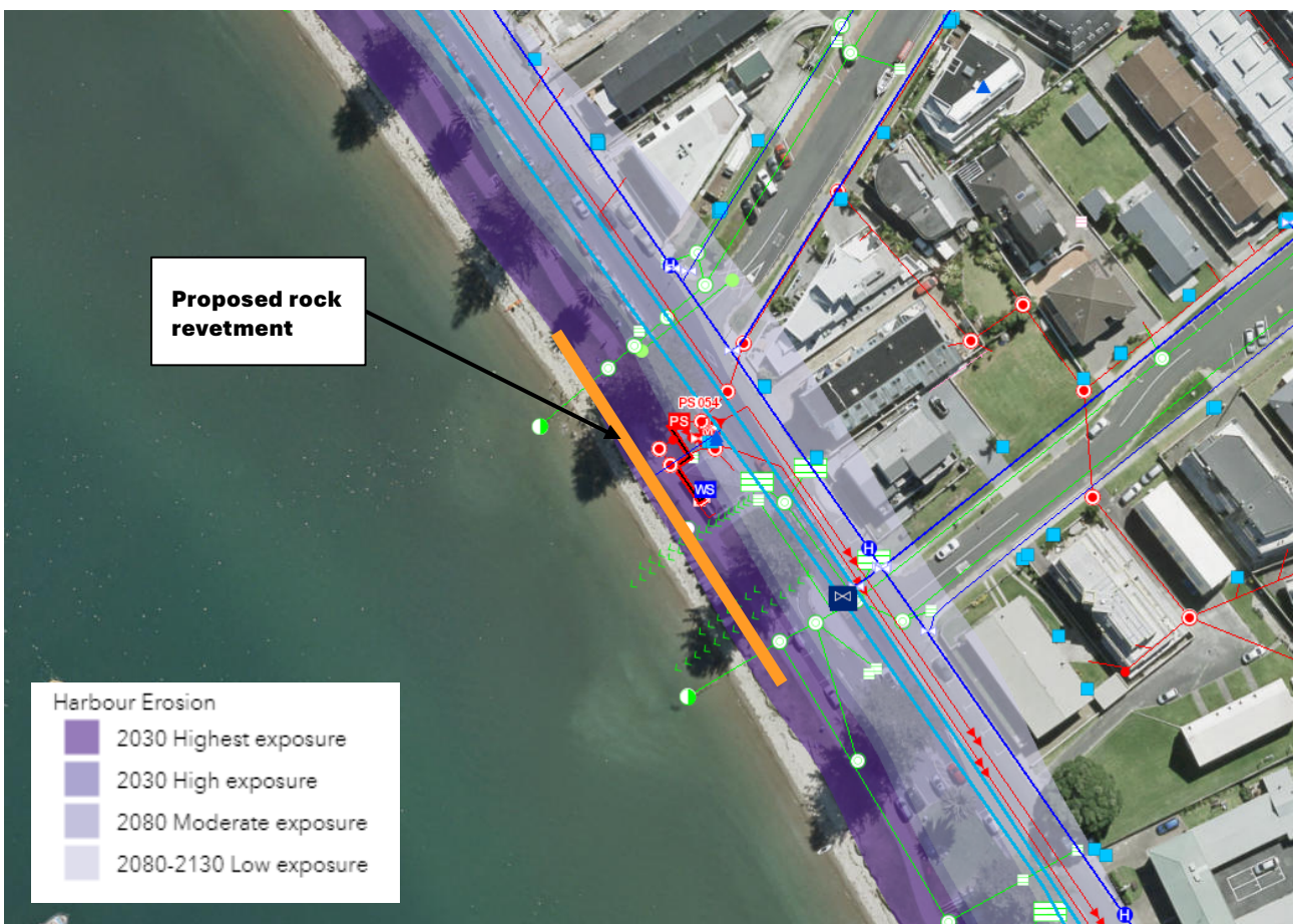
Figure 12: PS054 and proposed rock revetment location
