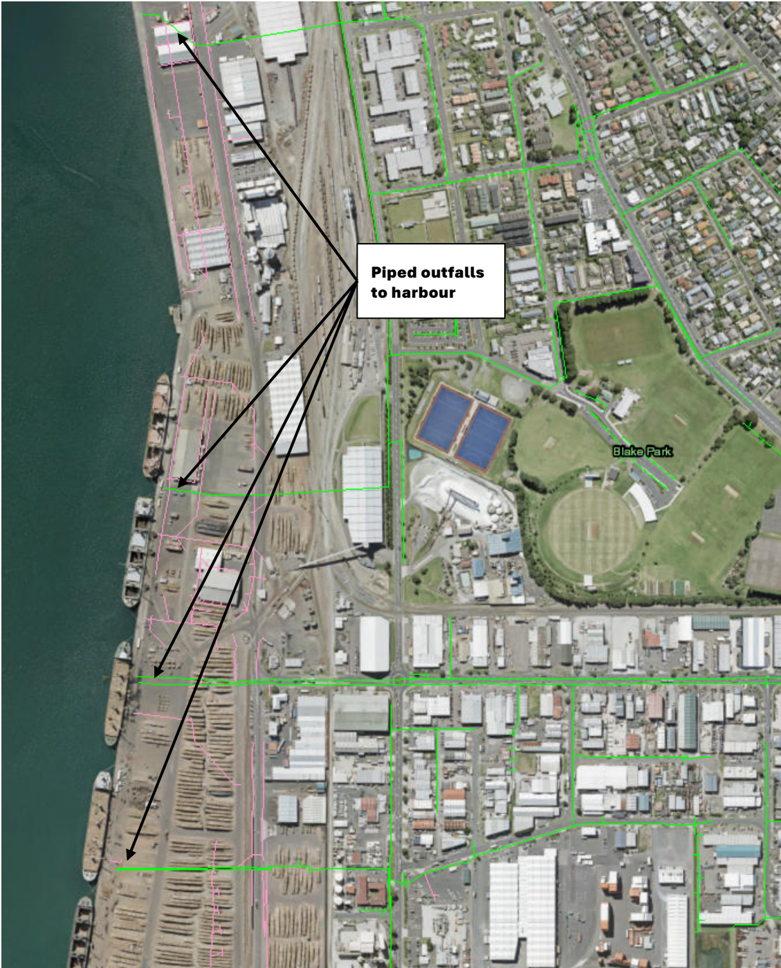
Figure 3: Piped stormwater outfalls to harbour
