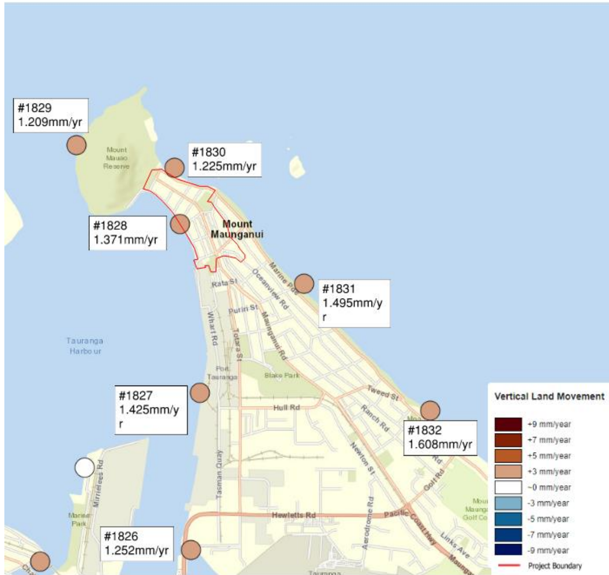
Vertical Land Movement Gauge locations and mean movement over 2003-2011 period for Mount Maunganui Area
