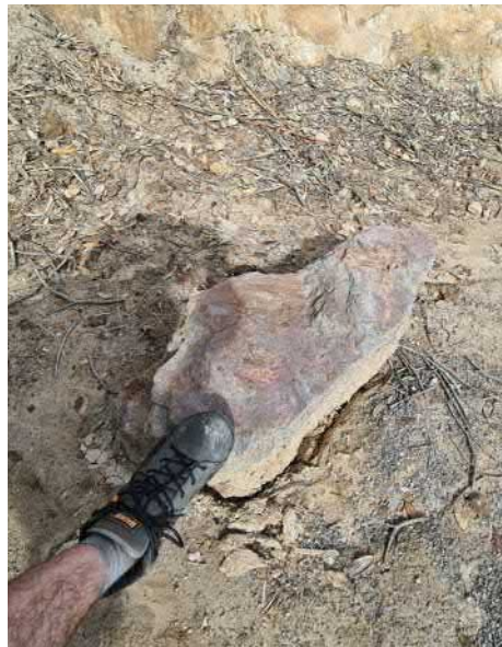
Photo 6 & 7; A recent rockfall from the actively eroding slope above the Western Base track.
