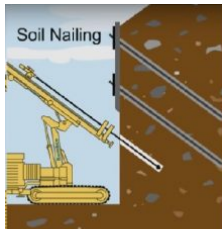
Figure 8:22: Soil Nailing Process
