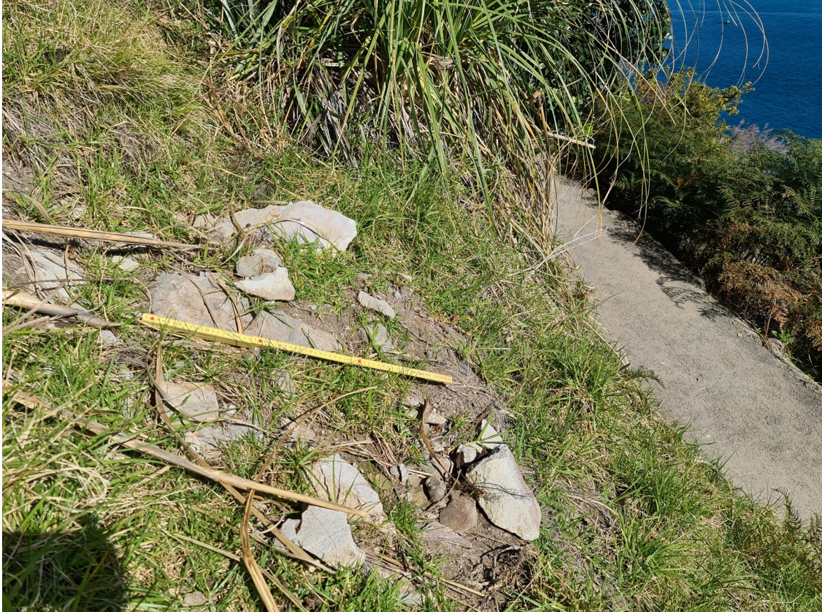
Photo 8; Rock resulting from a small soil slip above the Oruahine track.
