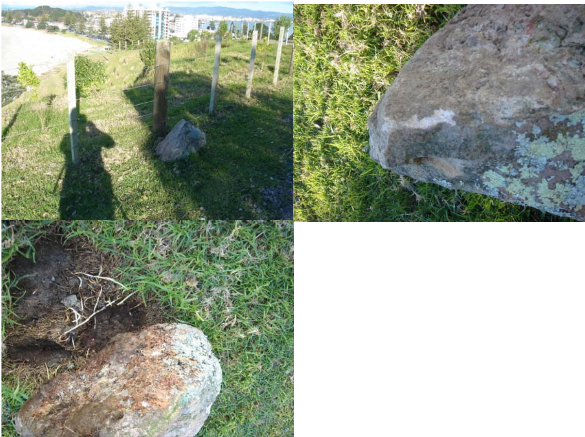
Photograph 2 (a,b,c); Surface boulder above slip 34 shows signs of impact and has decaying grass underneath.
