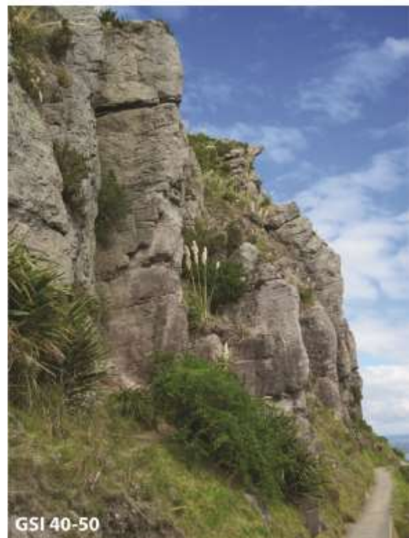
Figure 7: Distribution of the rock mass quality observed at Mount Maunganui and example of a representative rhyolite flow outcrop.
