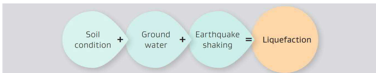
Figure 2.1: Three key elements required for liquefaction to occur - reproduced from MBIE/MfE Guidance (2017)
