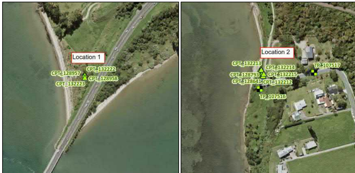
Figure 4.3: Two locations on Matapihi shoreline where 50MPa cones were undertaken adjacent to 100MPa cones
